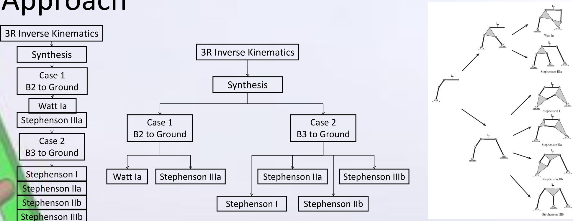
Our approach involved beginning with 3R planar chain synthesis. Our first approach involved using parallel computation for all of our calculations but maintaining series execution of the cases. Our second approach involved dividing the cases by dependency and assigning a processor to each case.
