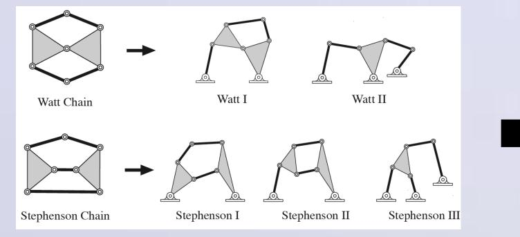
Once a 3R planar chain has been specified that reaches a set of goal positions, we can "program" its movement using mechanical constraints. The resulting mechanism moves with one degree of freedom.
